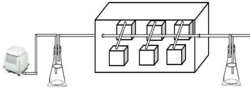
**Figure 1.** Schematic illustration represented the MVP fumigation chamber
