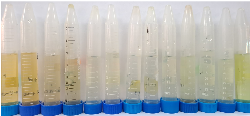
Figure 6. Color change of freshness indicator film for 24 hours at room temperature from pH 1 (right) to pH 13 (left)
